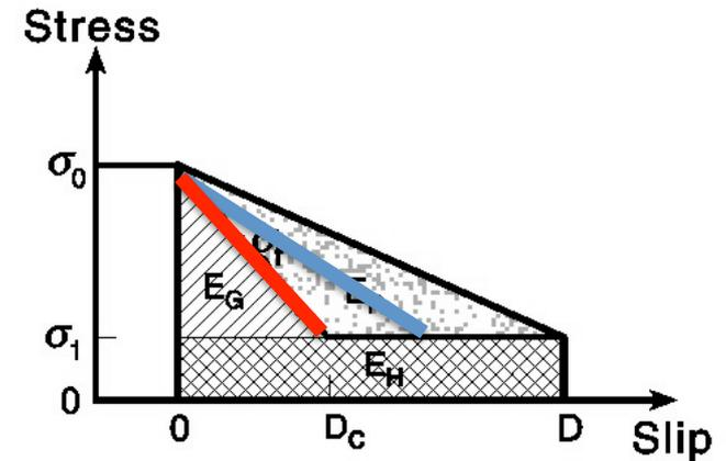
Fault constitutive model as well as rock mechanical properties affect HF induced seismicity. Acoustic emission measurement helps better understanding of fault model and numerical model calibration.
