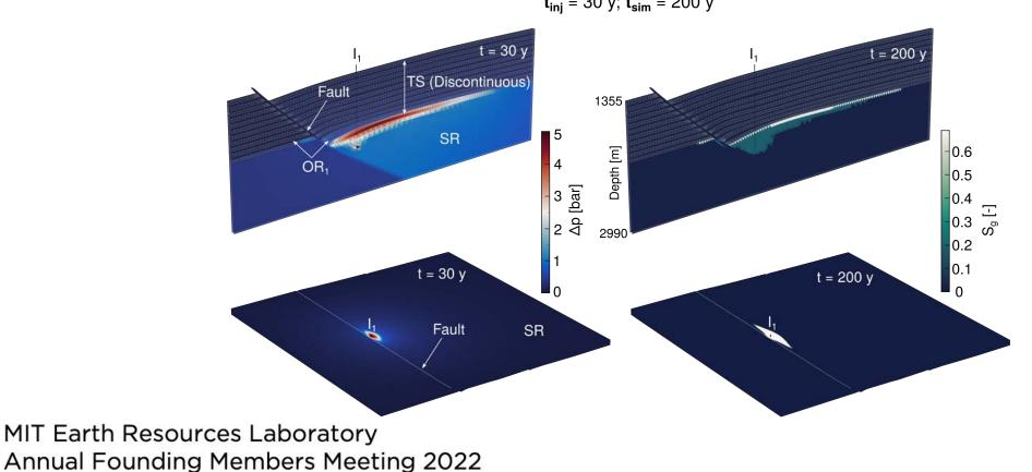
**CO**<sub>2</sub> injection rate: 1 Mt/y t<sub>ini</sub> = 30 y; t<sub>sim</sub> = 200 y
