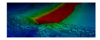
Thrust fault,  $\sim$  6 m elements, 2000 explicit steps, under 60 secs.
