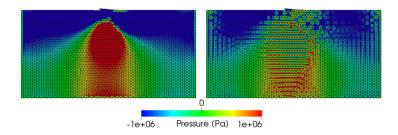
Pore pressure changes, 2D triangular element domain, following co-seismic slip on a thrust fault, with (left) and without (right) stabilization.
