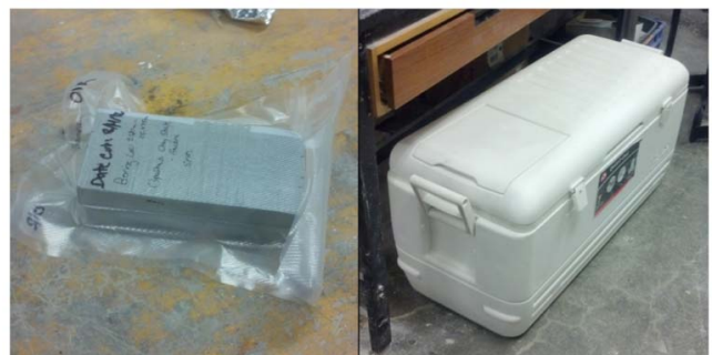
Figure 14 – Shale sealing and storage. Left: shale specimen is stored in vacuum sealed bags to preserve in-situ water content. Right: cooler container for added protection.
