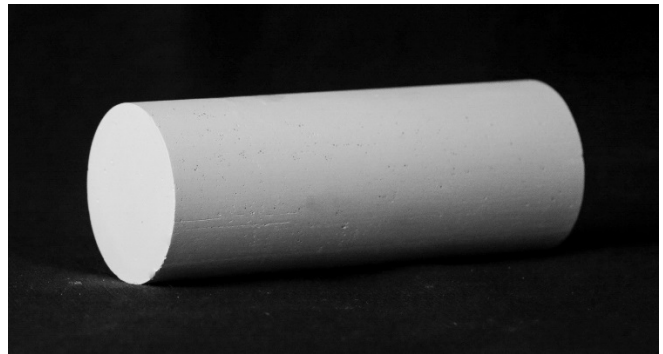
Figure 1. Gypsum specimen for core flood tests.
