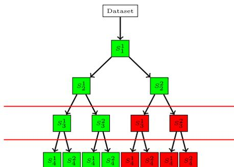
Fig. 6. Example of a BFS pipeline. The red horizontal lines indicate pruning points, which occur after the amplitude outputs of  $S_2$ . (For interpretation of the references to color in this figure legend, the reader is referred to the Web version of this article.)
