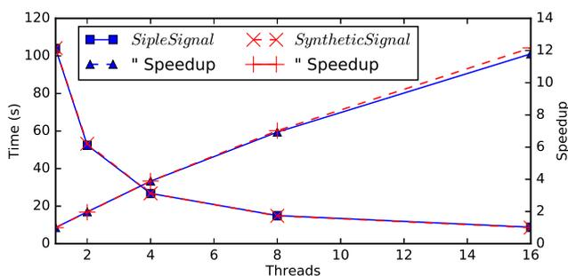
Fig. 10. Response time vs. number of threads using exhaustive BFS for *SipleSignal* and *SyntheticSignal* datasets in scenario *E1*. The right vertical axis shows the speedup relative to the single-threaded implementation.
